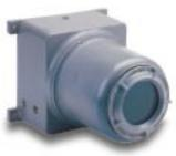
The NEMA 7 Housing is approved for Class I, Division 1, Groups C & D hazardous areas. It is for use with all General Monitors 2" and 4" wide controllers. The housing is provided with two conduit connections on each side, right and left. A reset switch is also provided on the right side for use when the controller(s) is ordered with latching alarms. The housing will accommodate one or two 2" (49mm) wide models. It can also house one 4" (98mm) wide model. Order P/N 10099.
